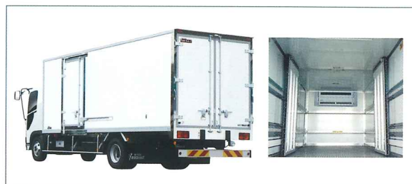
Two-Room Reefer Truck (Frozen/Chilled rooms)
